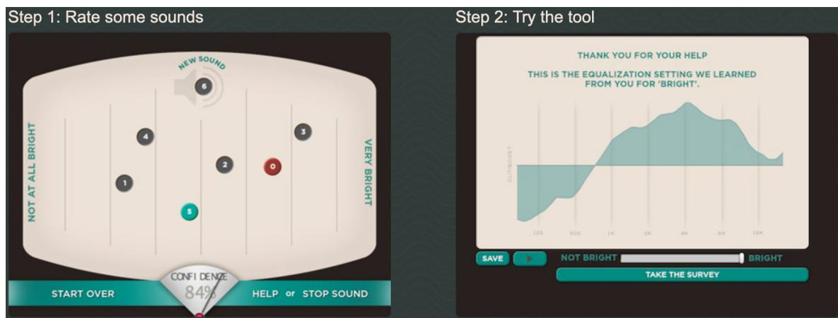
**Figure 3.** SocialEQ: an evaluative interface for controlling an equalizer. (left) The evaluation panel. Here, the user rates options to teach the machine a concept. (right) Once the machine has learned a concept ("bright", in this case), a single-slider control is provided to let the user fine-tune the equalization in terms of that concept. Screen capture created by the authors.
